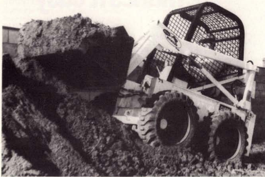
The Melroe Bobcat M-610 has a rated operating capacity of 1,000 lbs. and maximum lift height of 108 inches.
