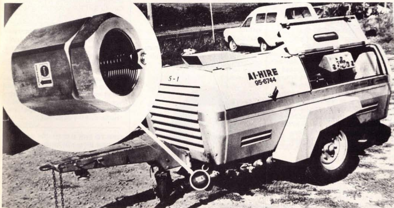
The Barfell Air Line Safety Valve fitted to a Hire Compressor.
