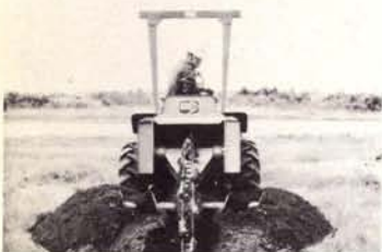
Double-auger digging assembly.
